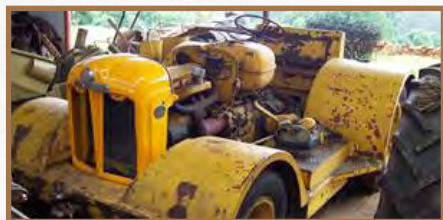
The only panel beating required was to the nose cone – shown here in JCB yellow, an indication of how the finished job should look.
