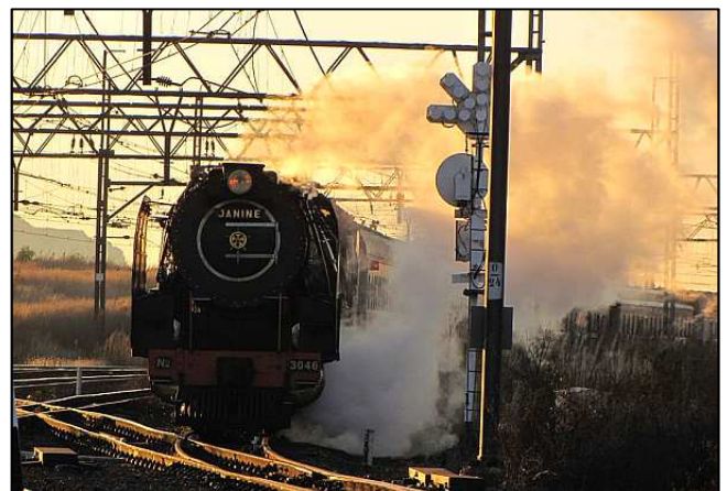
P192 - By the time the locomotive receives the green light to proceed on her journey, the effort invested to get her to this stage has already been in progress for 24 hours. In railway days, they were kept constantly hot and in steam for a week or more in between boiler washouts..
