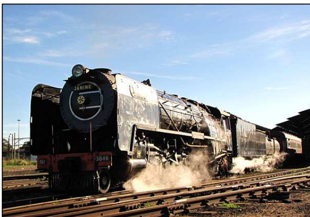
P191 - We use the western yard to assemble and couple up to the train. Before the train can depart, the auxiliary water tanker needs to be connected and the vacuum brakes need to undergo witnessed testing by the Train Safety Officer.
