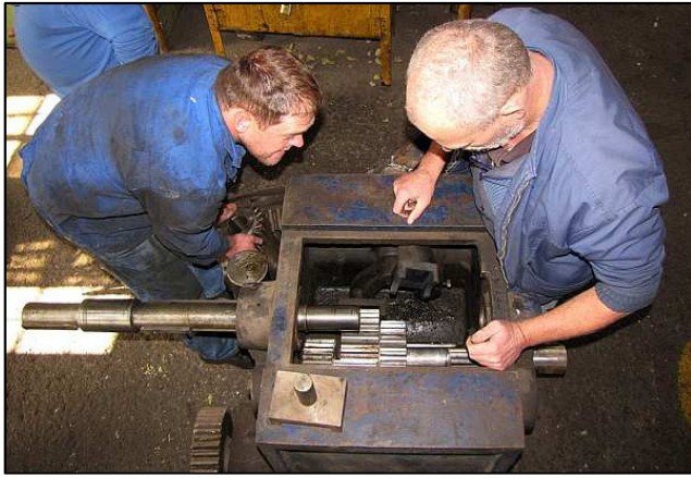
P175 - A valuable and yet hard-to-quantify skill is the ability to figure things out and make a plan with worn, incomplete and often undocumented machinery. These fellows are test-assembling a gearbox for the locomotive wheel lathe project. The talented gentleman on the right passed away suddenly less than two weeks later.
