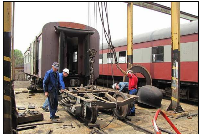
P164 - Coach bogies also need to be inspected and serviced at regular intervals – and this is usually done in the 15M shop or surrounds. This one has been rolled out to have the coil springs uprated as the caboose was riding tilted with the weight of a newly installed generator set inside.
