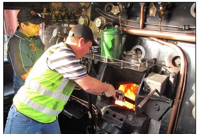
P174 - Most of our trains run with a 'third man' on the footplate who assists the fireman and gains experience in firing. In the early days of his training, Simon Bennett is seen being taught how to fire to the right corner via the awkwardly inset 15F firebox door.
