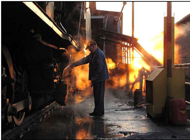
P189 - While the fireman cleans and rebuilds the fire, the driver will go around the locomotive with a can of oil to refill all the oil cellars, and to lubricate the moving parts. Here, Senior Driver Chris Saayman is filling up the oil cellar on a Bissell truck's radial slide.
