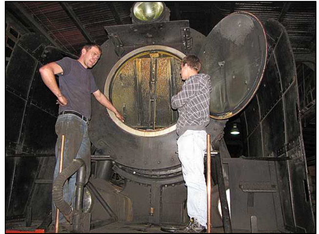
P176 - We hold training sessions at intervals. Here a keen young man is having the drafting arrangements of a self-cleaning smokebox explained to him. He can now commission and decommission a locomotive on his own.
