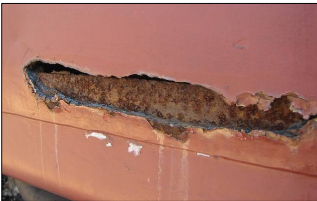
P09 - Naturally, being stored in the coastal region means a lot of rust. Thankfully, 'Dusty' wasn't stored directly at the Shepstone Coast, so the tin worm isn't as bad as it could have been. The coach boys will need to use the techniques they learned by patching up the Sandstone Sleeper Coach to fix this lot up.
