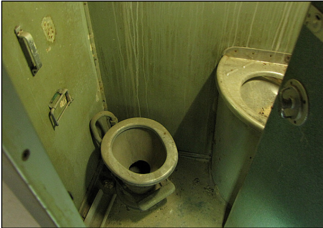
P07 - Dusty's toilets are intact but derelict. This coach will be the first of our day sitters to be fitted with porcelain toilet bowls. We are also considering using this coach as a test bed for our planned on-board cess-tank systems to gain experience before converting the sleeper coaches.
