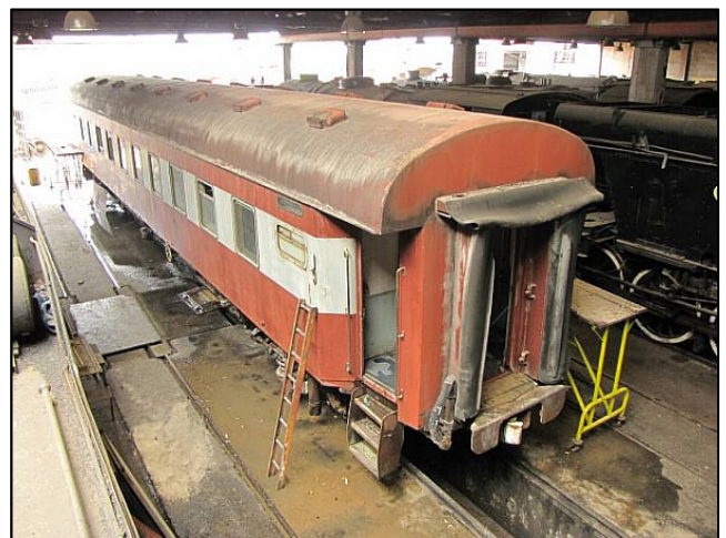
P12 - This is what 'Dusty' the Semuma Coach looked like after her first high pressure WAP washout in May 2012. You can see how caked the roof and crevices were, and where the evil rust has taken a hold.
