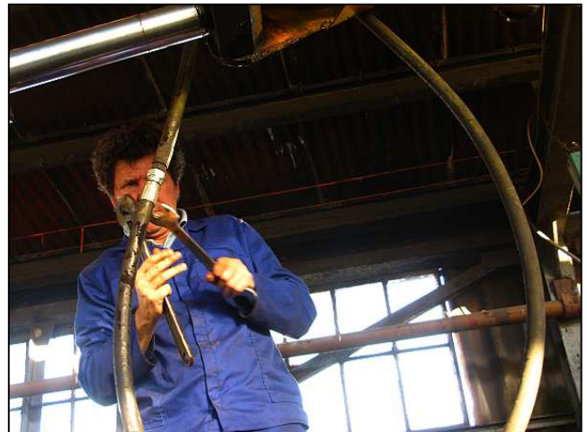
P16 - With the gripping of incompressible objects in the grab, the hydraulics took some strain and one of the hoses burst. It was the hose to close the grab. Alan quickly couples the hoses together to form a bypass loop and the clamshell would remain open for the rest of the day.
