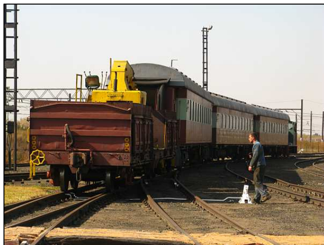
P24 - The short train is almost clear of the points and is just about to be called to a halt. Although it was broad daylight, this shunt move was still performed with radios.
