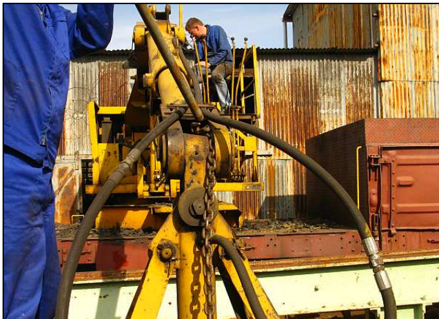
P31 - When the grab was previously used to hoist the Class 12AR bogie axle, someone had unthinkingly looped the octopus chains over the pivots to make a shorter sling. (They should have been looped around the impulse bar.)
