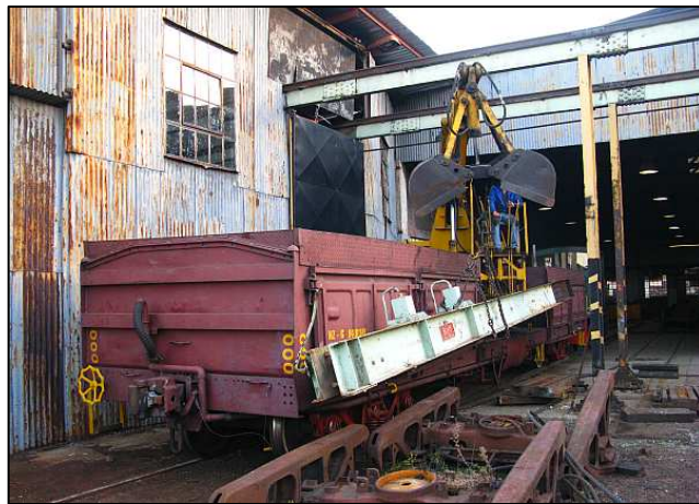
P42 - The Swager's top section was dragged into alignment with the grab via chains and then hauled up 'side-saddle' against the wagon. It was being slowly shunted out at this point. The nice thing about playing with an old DZ wagon is that you don't have to worry about the paintwork so much.
