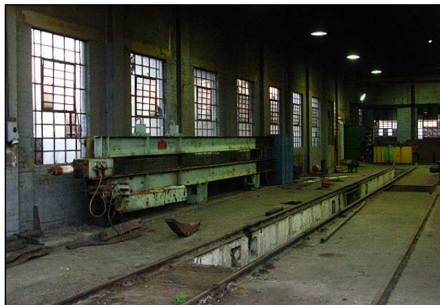
P44 - Dear ol' Swager, finally laid to rest – but to work again in the future. The machine is operated from the side but there is plenty of room for two workers to turn corners with boiler tubes which can be over 6ft long. Where the blue cabinet is will later become a tube storage rack area.
