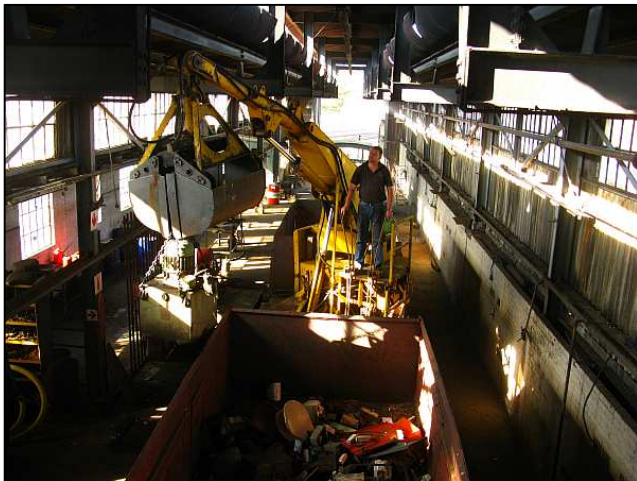
P15 - The high sides made lifting the bigger items more awkward as we couldn't get enough height in the boom under the roof. There were some near misses with the lights too. For this move, the train had to be shifted gently for an extra last few inches clearance below the roof truss.
