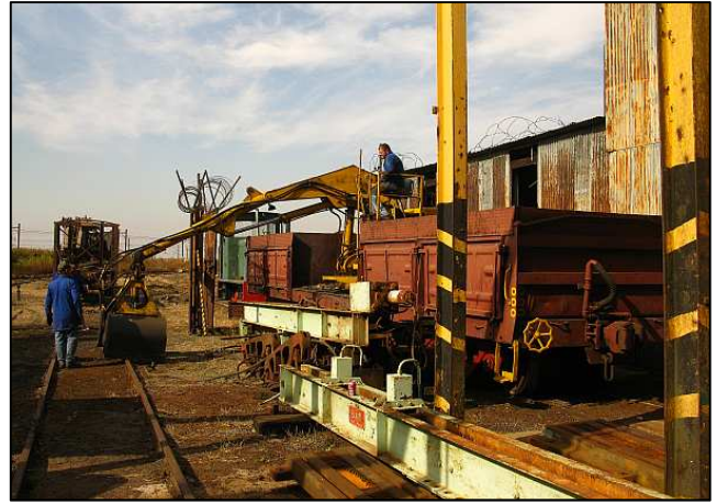
P30 - This picture is educational as it shows the full reach of our useful coal handling wagon. The bucket was placed firmly on the ground in an attempt to relieve the weight in the suspensory pivots and hopefully to release the jammed chain. It didn't. So, out came the wedges and gwalas...
