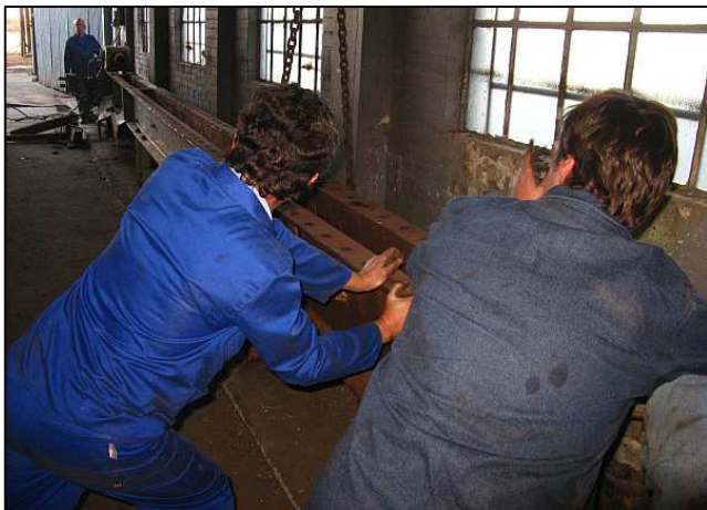
P41 - A synchronized shove to get some momentum going. The final move was a long-levered swing using the ram base as a pivot. I have frequently cursed the uneven, pitted flooring of the workshops. Now I know where those chips come from – we added a few ourselves today!
