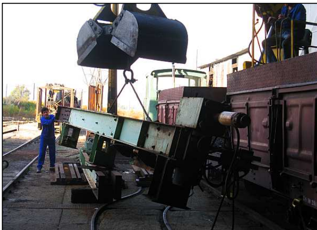
P33 - It took three attempts to find the center of gravity and to slowly edge that heavy ironmongery away from its resting place. It is fairly easy to guide a suspended load – but it can be dangerous because even though the weight is suspended, you still have the full inertia to contend with – which can crush extremities if you are not 100% alert.
