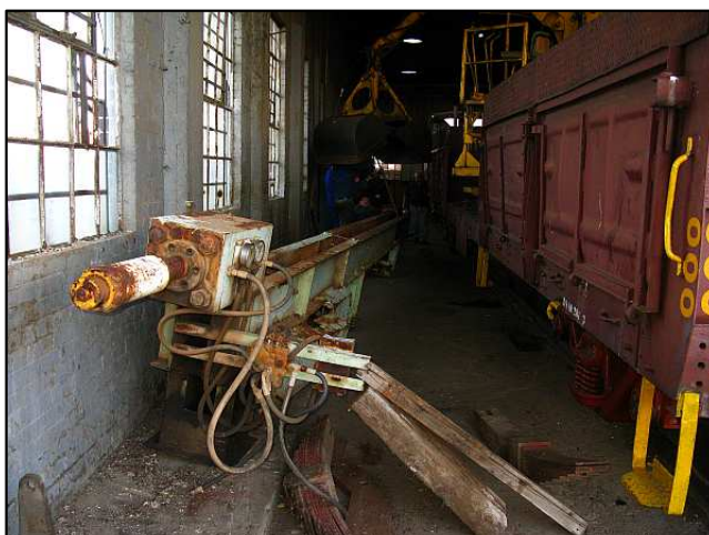
P40 - The coal grab's clamshell cannot be rotated, so the slings could not be traversed without smashing a window out. So we 'landed' the Swager ram-end first and braced it while adjusting the slings. For safety's sake, no one was allowed to go between the wagon and the tilted machine.
