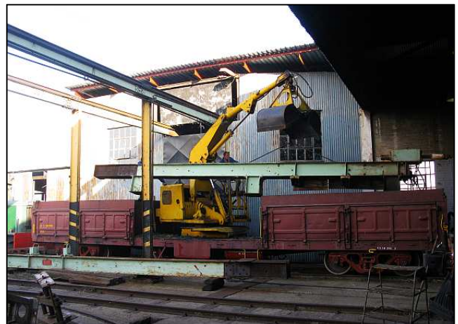
P34 - The final lift for the Swager base section with the shorter slinging took place out in the yard again, as that was the only location where the coal grab's booms could extend high enough to swing the load over the two bunkers.
