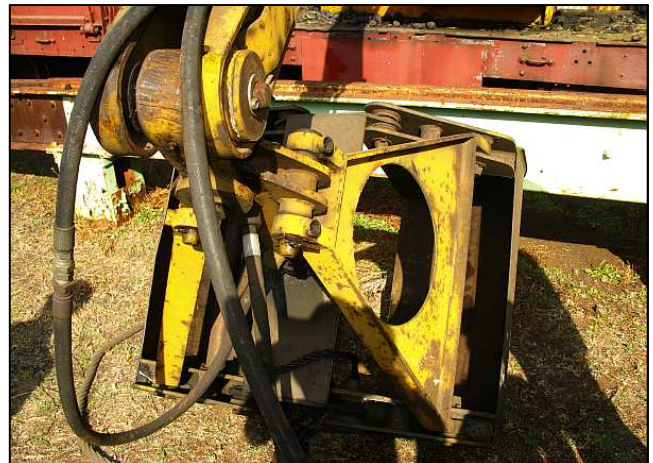
P32 - Suggested by you-know-who ☺, an unusual view of the clam shell's bucket. It was lowered and tipped against the ground and then the boom rotated to offset the weight in the pivots – it worked and we got the jammed chain out.
