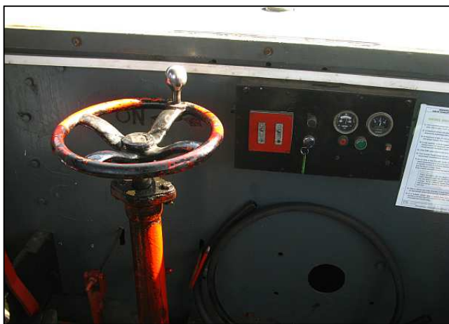
P27 - 'Andrew's' brake wheel stand with the tricky left-hand thread. (Note the left arrow.) The voltmeter shows why the battery keeps going flat. Just under 13 volts is insufficient to charge a calcium LA battery – the Lucas ACR alternator on a slow running diesel motor just isn't up to the task.
