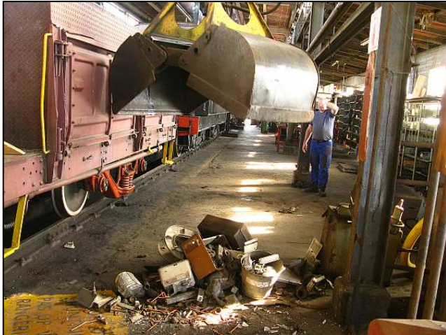
P13 - This is about the fourth load. We could have dropped the sides of the bunker and tossed everything in – but why bother ... as we had some heavier stuff to hoist over the high sides anyway. (The checker plate scuttle boards above the DZ-style drop-doors are not removable.)
