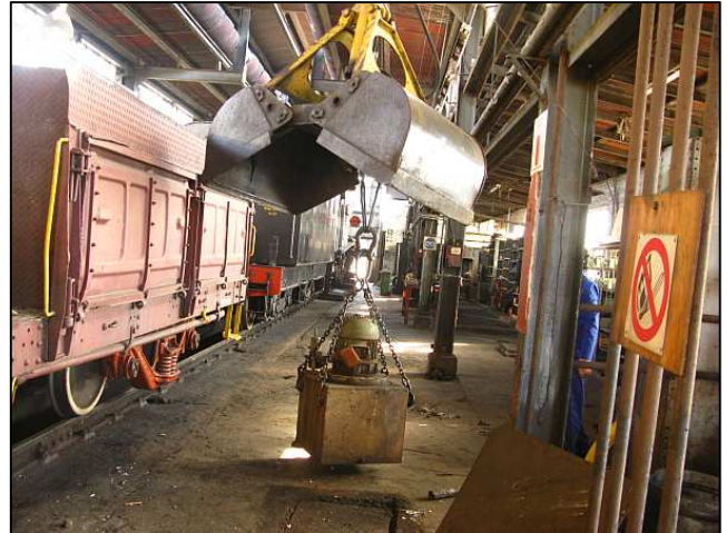
P14 - The hydraulic pump pack is being hoisted out. Rather than scrapping, this unit was being relocated into the 15M shop for repairs. The motor has been damaged by water ingress from the leaky roof. (We use this machine to test the integrity of newly repaired superheater elements.)
