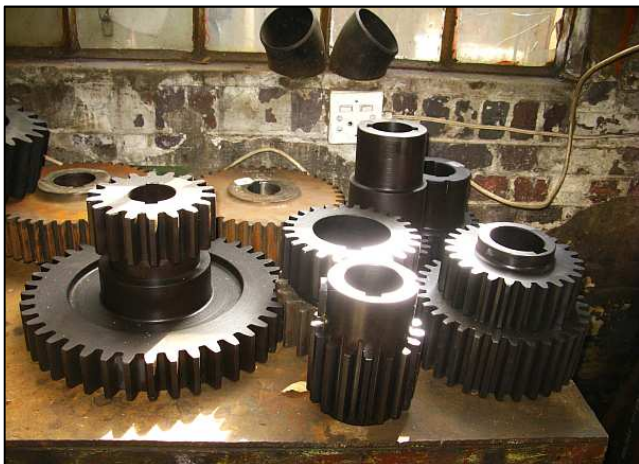
P45 - The wheel lathe gears have been returned from their hardening process and reassembly of the two gearboxes should be starting this week. We plan to contract the electrical work out and if it is done in time, we COULD have the wheel lathe running for the Depot Open Day on 26 July.
