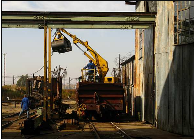
P29 - A great start to the job – you can see the octopus chain swinging from the grab – it had jammed in the grab's pivots. This photo shows the obstacles and walls restricting both the arc and the height of the boom operation, making this technically simple job into a proper 3D challenge.
