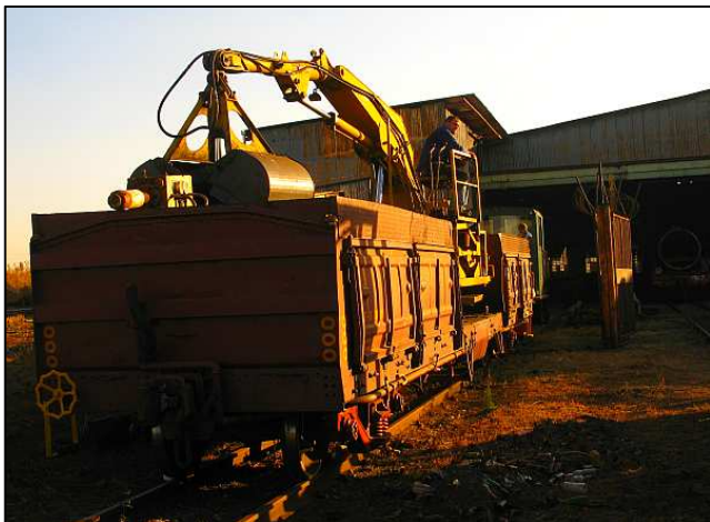
P37 - Getting the asymmetric load through the heavy gates was going to be a problem and you can see by the golden light that it was getting late. Note the use of the open grab to force the ram end down to prevent tipping.
