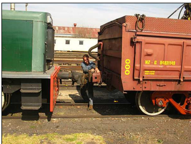
P25 - The wagon's coupler had ended up pushed slightly out of alignment, the effects of which are worsened by the sagging 'alliance coupler' on the diesel. Carefully standing on the driver's side, Jeandre yanks the coupler over.
