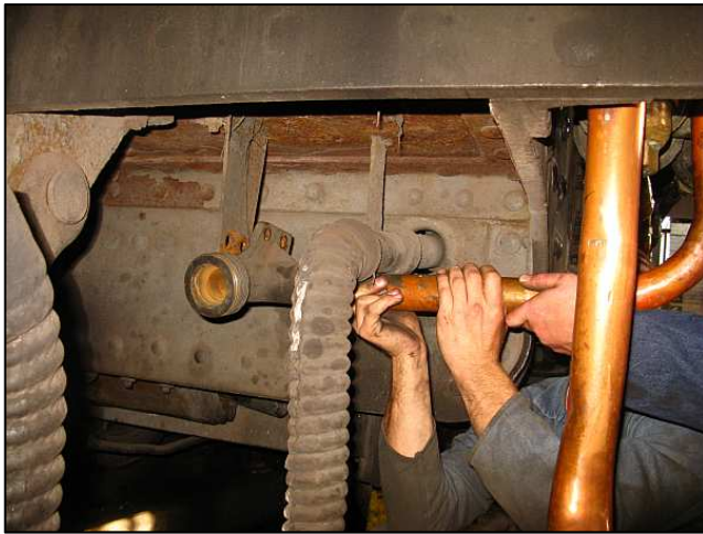
P25 - Here is the other end that needed to match up with two bolt holes to be engaged. This is where the flexible water hose from the tender is attached to the locomotive. The ribbed rubber pipe is the train brake vacuum pipe.
