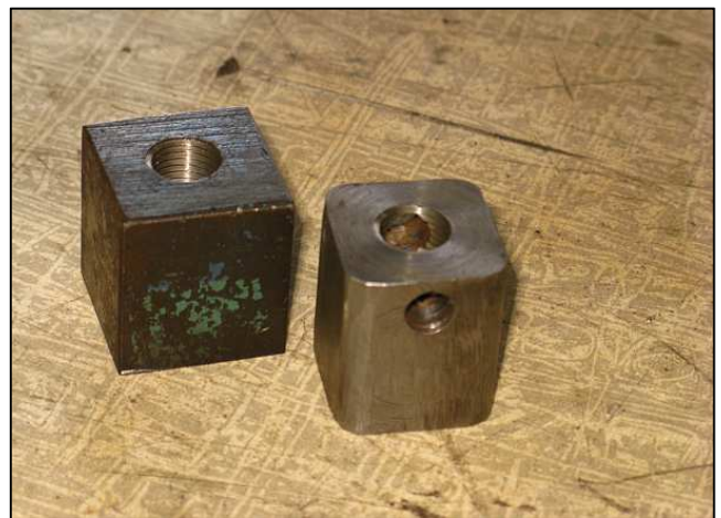
P06 - New shank blocks were machined to help eliminate excess play from the system. Unlike with the originals, the valve kick lever will only be allowed to operate through a 90 degree arc, so the system must not have any free play.
