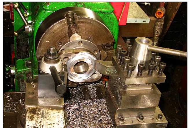
P18 - Dawie initially did some VERY judicious grinding of the new welds with a small angle grinder. Then James cut down the new gasket surface on the TBS lathe.
