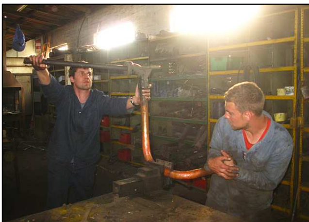
P29 - 'Swak Hart' Viljoen applies a bit of leverage to apply more grunt with an optimistic Jeandre trying to hold onto the other end without extension of leverage. This 3D bending process usually has to be repeated several times to get a good fit.
