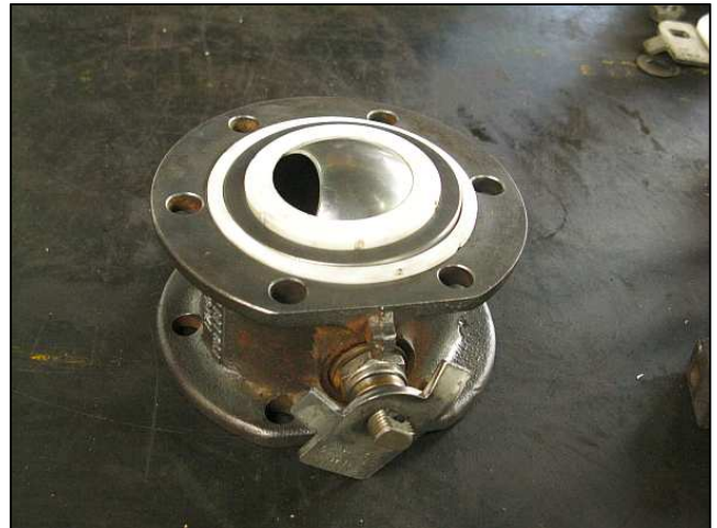
P04 - The vintage bronze water valves are being replaced with PTFE-seated stainless steel ball valves. The leaky originals waste the tender's water, but also dangerously distract the fireman as he has to look down and kick the loose-linked lever back-n-forth to find the elusive 'off' spot.
