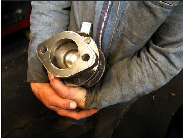
P13 - Here is a view of the assembled ball valve about to be installed for a trial fit. It was already known that the valve would be about 25mm longer than the existing and the pipework would need to be modified slightly. But our young steam-nutz were just about to get a nasty surprise!
