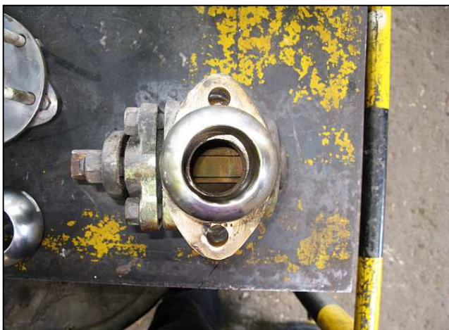
P05 - The bore in the new ball valve is 6mm wider in diameter than the original valve bore.
