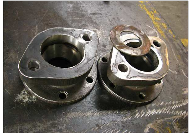
P16 - The flange on the right had a rebate carefully cut into the bore to accept the collar washer. The left flange (for the copper pipe of the water riser) did not need any modification. The flanges are quite chunky but will be less prone to distortion as the originals can be.
