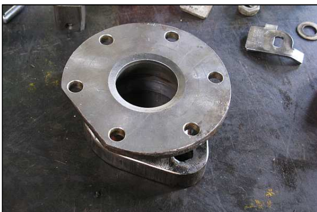
P11 - These new flanges were custom-made by Jeandre's dad. They are very close-coupled to the valve body flange, to keep the length of the new valve assembly to be kept to a minimum. The whole new assembly was able to fit in a length only 25mm longer than the original cast-body valve.
