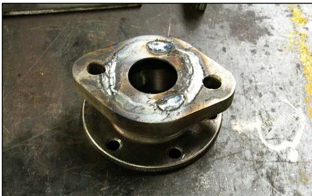
P17 - The same flange after welding. The mismatch on the RHS means that we mainly lose the advantage of the wider-bore water valve, but we will still utilize the positive action and better sealing. But even if we didn't match up the gasket face, the mismatch still would have been there.
