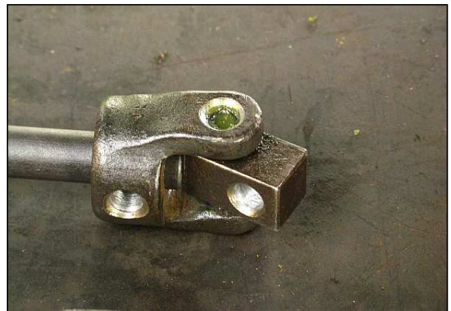
P10 - A close up of a universal joint being overhauled. These joints are being repurposed from old turret valve spindles, which usually only have one universal joint each. The yokes and die blocks are being drilled-out and pinned together with spring steel pins to eliminate all free play.
