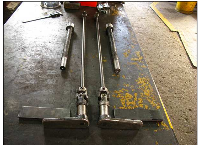
P08 - To move the kick lever from the floor to the wall required an extra shaft to be made with a universal joint at each end. The short shafts shown are similar to the originals which pass loosely through the cab floor to couple onto the valve stem via a noggin and socket arrangement.
