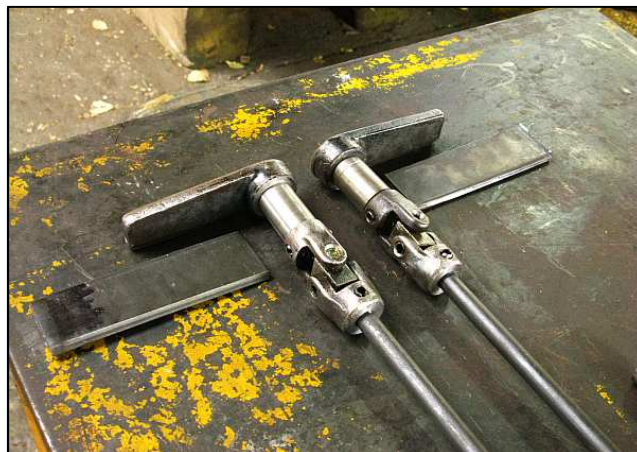
P09 - Detail of the kick levers mounted onto new stubby shafts, each running within a machined sleeve. The sleeves will be welded to the two bars which will protrude from the cab wall and will also support the quadrant stops. The tubular sleeves will also have grease nipples fitted.
