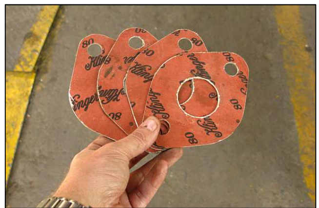
P12 - The gaskets made in advance for the new flanges. This is Klingerite. As the new valves use stem seals, they do not need a bolted-upper cover as the originals do. Those old top gaskets are frequent sources of failure if not fitted 100% correctly or the injector allowed to blow steam.
