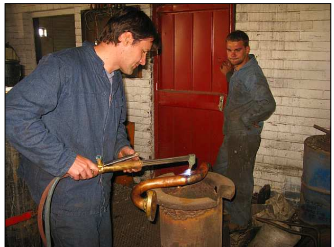
P28 - Dawie heats up the copper to dull cherry red before they dunk the hot pipe in a wheel barrow full of cold water parked right outside the door. This process is 'annealing' and it softens the copper pipe prior to bending - rendering it more malleable ('bendable') and less likely to fracture.
