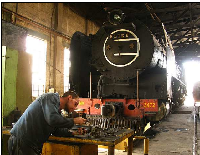
P21 - This was a fiddly job with SIXTEEN bolts all needing to be precisely cut down and their threads cleaned up.
