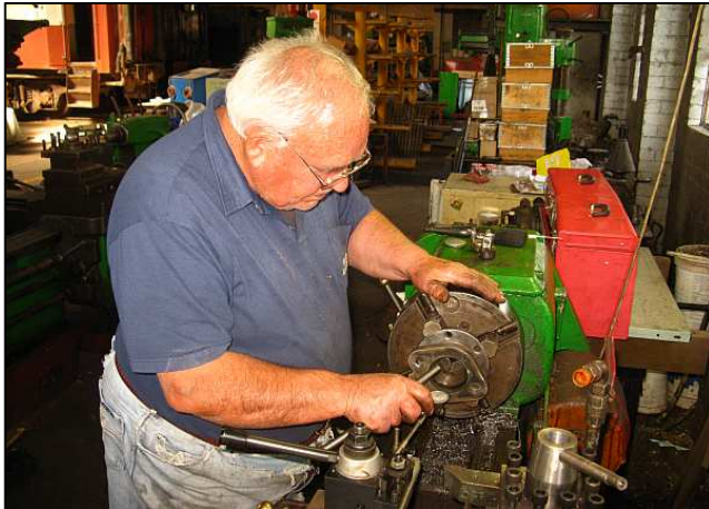
P15 - We could just assembled the set, but the RHS inlet would have been prone to gasket failure due to insufficient mating surface for the gaskets – even under the passive pressure from the head of water in the tender. James machined a groove to fit a repurposed collar washer.
