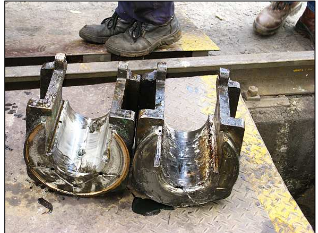
P02 - The damaged bearing is on the right. On the intact bearing on the left you can clearly see the three holes and the milled grooves that dispense oil to the thrust face.
