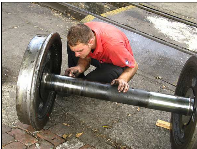
P09 - They say that if you can catch your fingernail in a groove in a car's brake drum, it needs machining. Well, this axle DEFINITELY needs a spin - Jeandre checks out the grooves. A pity, as this axle had never been turned-down before. The RHS shows the diameter as first made.
