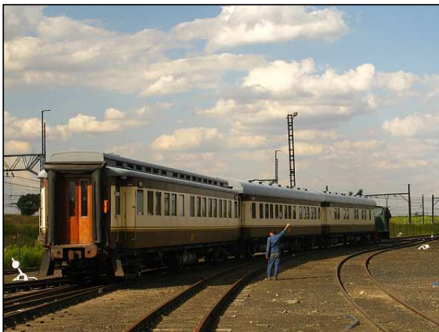
P05 - Alan gives the confusingly-named 'forward' signal. This shunting hand signal actually means 'move away from me' and it is always with reference to the position of the shunter, not the position or orientation of the locomotive. The Hunslet locomotive is actually moving backwards here.
