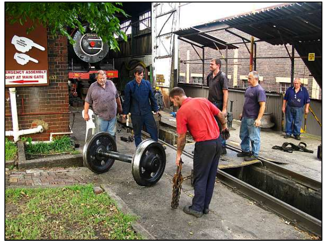
P08 - While the shunting was in progress, the other fellows managed to get the damaged axle off the ash pit rails without losing any fingers or toes. Jeandre has just caught and brought in a 'Ferrous Octopus' chain for hoisting.
