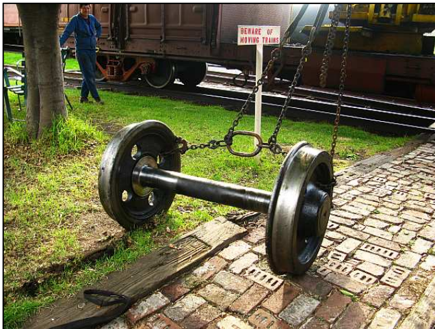
P15 - Here! I say, Sir! Please keep off the grass! The first part of this operation was a simple drag to get the axle under the range of the boom to be able to get a safe lift. You can see what a locomotive wheel can do to your lawn!
