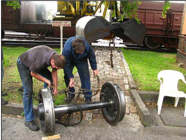
P13 - Dawie and Shaun hook up the four-legged 'Ferrous Octopus' – which just about fitted because of the holes in the wheels. We do have proper spreader bars downstairs for the bigger counterweighted stuff.
