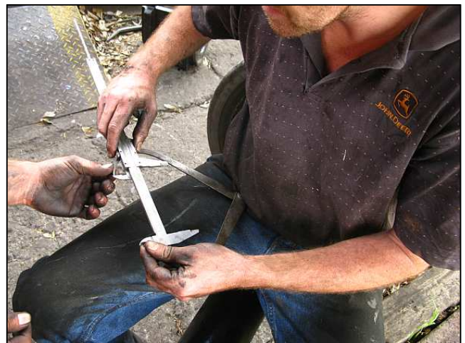
P10 - Capturing the approximate depth of the grooves with a set of callipers and a vernier. The axle journals will need to be turned down on both sides and both bearings to have their white metal re-poured and machined to suit - otherwise you end up with a canted bogie.
