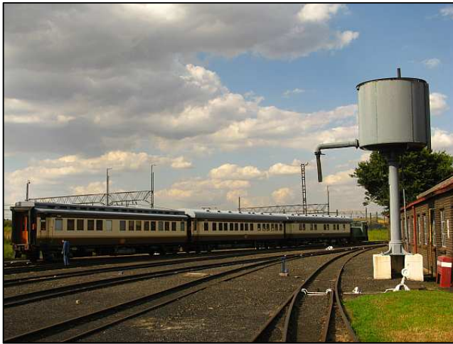
P07 - The entire three coach train fits in easily behind the points. Much more than another coach length and the train would have needed to be split as the little Hunslet pluggers does not have the weight to safely stop the coaches on the downgrade into the turning balloon beyond.
