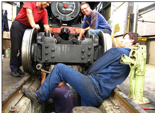
P04 - The left side (Right in the pic) came out easily enough. The nut actually span right off by hand on the decent threads after the initial 'set' had been slogged out. But the other side was binding – and 'Swak Hart' Dawie hams it up here for the camera.
