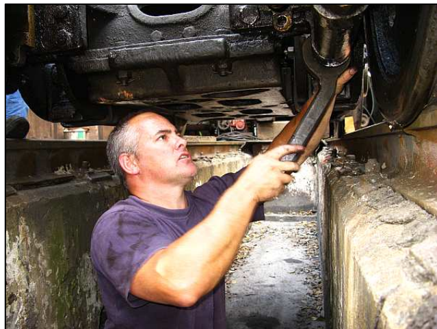
P02 - Grimacing in concentration (Trying to remember which way the nut turns?) Michael applies the slogging spanner. These spanners are intended for whacking to spring tightened threads loose, and the slender handle is also intended to be slipped into tubing for extra leverage.
