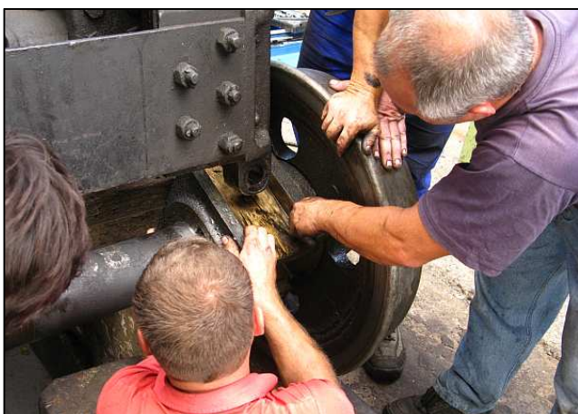
P15 - The heavy brasses are rotated on the axle to clear the keep bolt eyes – and both of them have to be turned around at the same time, preferably without denting the horn faces. This is a deceptive operation as the axle takes the weight, but not the inertia, and it is easy to rotate the bearing too far and suddenly lose your oily grip.
