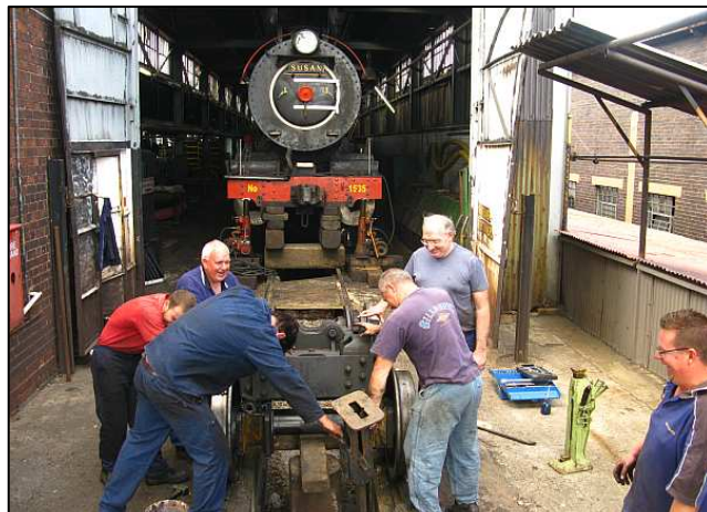
P14 - Dawie and Michael lift the jack away from the blocked-up bogie before the axle could be rolled out.
