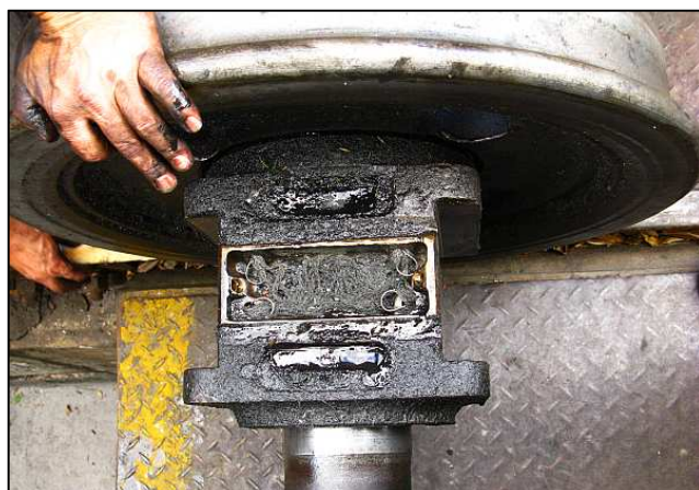
P18 - Another view of the crown reservoir. It looks empty ... which is normal as the wicks continue to deliver oil even when the locomotive is out of use. (All wick-type oil cellars auto-feed until empty.) The fault turned out to be elderly axle oil socks that collapsed under the bearing journal – and it is those socks that provide the main lubrication when the engine is in motion. This axle was relatively new and did tend to a bit run warmer than the trailing axle anyway.
