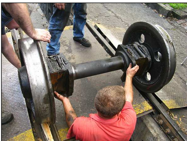
P17 - The axle was rolled over the walkway and was scotched-down by Aidan while Jeandre continued to stabilise the two bearings from accidental rotation. (Even though they didn't have far to fall – the purpose of this location.) Thus, you get a view of a complete loco bogie axle and its two 'plain' bearings in situ on the axle journals.
