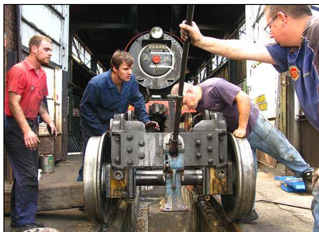
P10 - This is the first stage of a two-stage jack, block and then jack-some more operation. You can clearly see the brass axle boxes being gradually exposed as the frame lifts relative to the axle.
