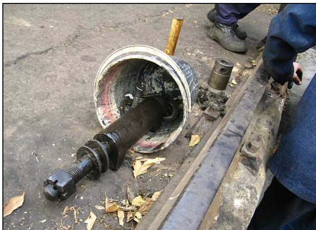
P03 - Before the bogie could be jacked, both of the front axle's tubular axle keeps needed to be removed. These span the bottom of the axle horn space under the axle bearing. In SAR steam practice, the term 'Axle Keep' is often also used to refer to the lubrication hardware such as the removable oil sock boxes and grease pad holders.
