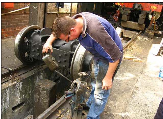
P09 - The green 'click clack' jack was changed for a 'Simplex' jack with a safer (less worn) ratchet and a lower lifting arm. It hasn't been used for a while, so Simon applies the slippery stuff before it is put into service.
