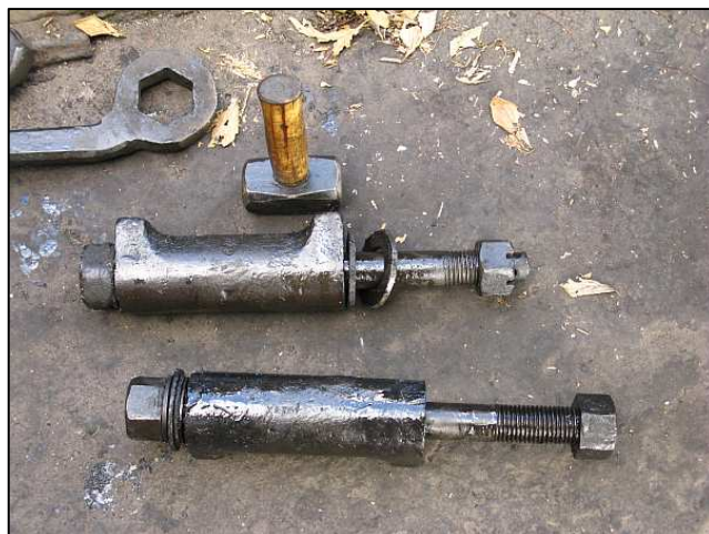
P08 - The tubular keeps exposed. The keeps are cast with generous ends to allow them to either be mildly skimmed down or to shimmed-up to suit different axle horn spans. They are not intended to be the primary adjustment for longitudinal axle box clearances though, as they would pinch or spread the axle horns out of parallel.
