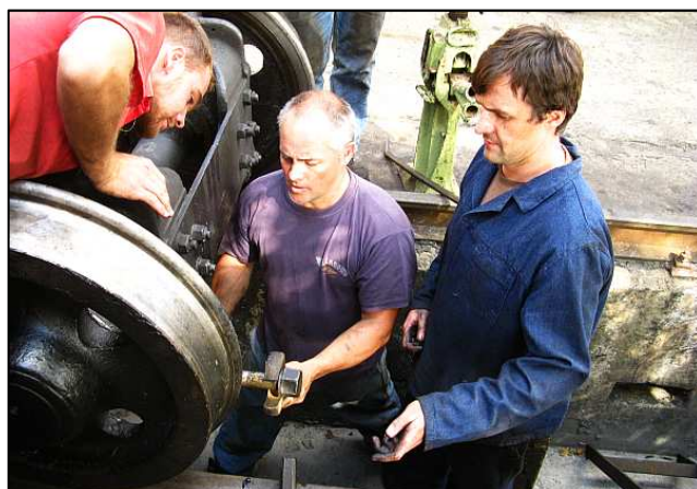
P06 - Due to misalignment, the long keep bolt was binding – even with a spanner used to drift it out under the head.
