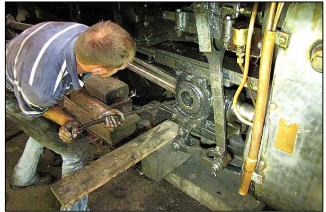
P16 - It was hoped to be able to push the piston (and crosshead) forward to disengage the small end and let it drop. This would tilt the connecting rod down out of the way of the slide bar. But, without the wrist pin in place, the connecting rod was tilting slightly outwards under its own weight and the small end of the forging engaged by friction.
