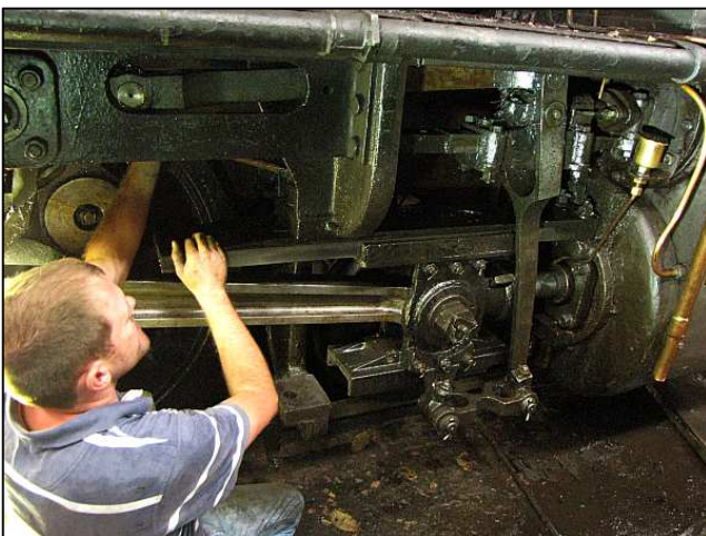
P11 - The upper bolts at the back end are easy-peasy to reach – with the fingers. But there isn't enough room to swing a dead depot rat behind the motion bracket – we lost time trying to find short cheaters to match the wrench.
