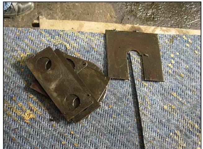
P22 - Here is a pile of the shims that were removed. Today's project would be to pack the slide bars away safely and to measure up for a new shim for the lower bar. The new shim would have to be between 4-4.5mm to allow for that amount of material that was taken away.
