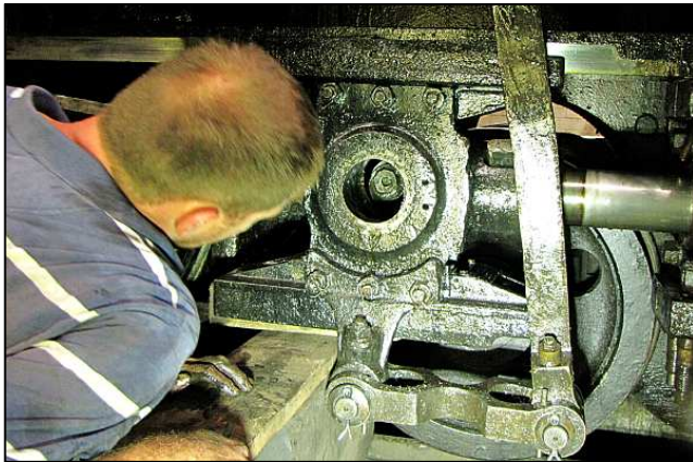
P15 - The gudgeon, or wrist pin, came out easily from the small end's bronze bushing, but then it tilted and started to jam between the crosshead and the bogie wheel. Fortunately, the last few drifting whacks weren't at full capacity (More like steady nudging) so we didn't have a totally wedged pin in there.
