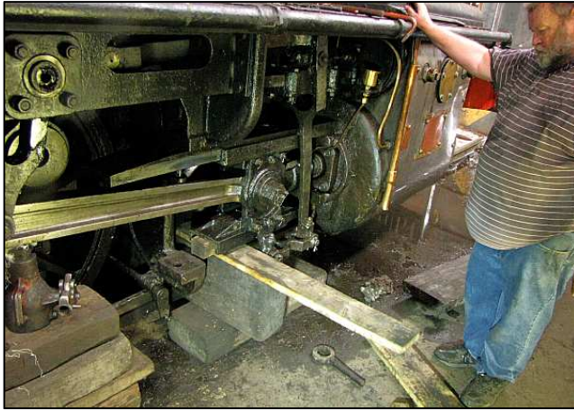
P13 - Here, you can see the error. The connecting rod is in the upper front quadrant and obstructs the slide bar from moving rearwards. Sigh. The fellows had to block up the cross head to prepare to remove the wrist pin. (Small end.)
