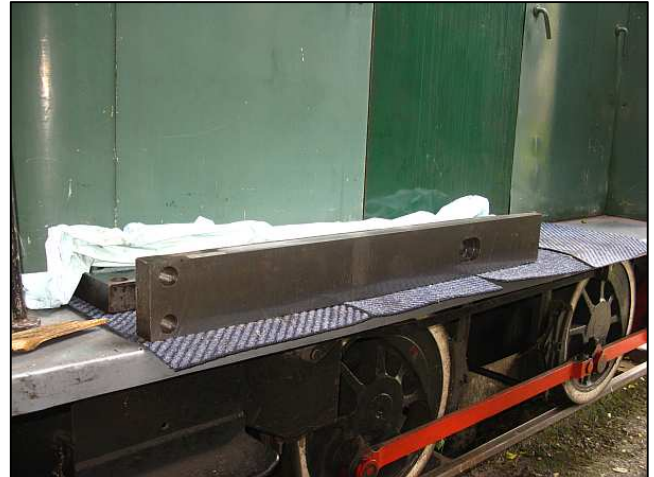
P20 - A closer view of the newly machined and freshly oiled crosshead slide bars – this is the plain-topped lower bar.
