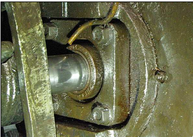
P09 - With the crosshead unsupported, it would not be a good idea to move the locomotive to shift the pistons, due to potential damage to the glanding hardware and the garter rings. Unfortunately, the shunters didn't think about putting the connecting rod in the lower quadrant, so it later got badly in the way to remove the upper bar.
