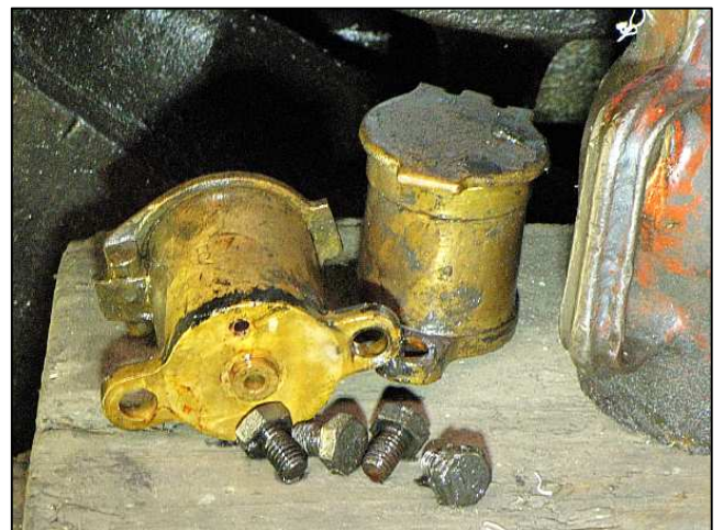
P12 - The two oil cellars were removed once the back bolts were loosened. You don't often see this underside view of a direct discharge oil cellar. (i.e. : Without a drip feed pipe.) These were carefully locked away, as all our brass stuff is.
