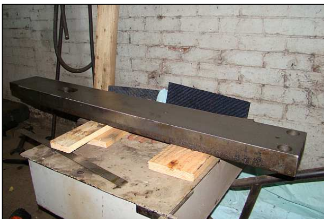
P23 - An already SMUDGED upper crosshead slide bar prior to being fitted on Fri, 21 March (Human Rights Day). You can just see the two oil holes into which the oil cellars feed. (Pic P12) This bar 'only' needed 1mm machined off.
