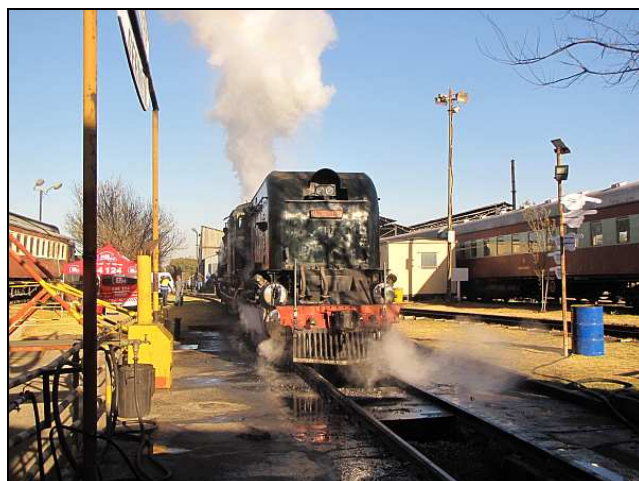
P38 – After a brief session of fire cleaning and lubrication, the GMAM rumbles away to the crossover points. She's quite light-footed for such a big engine and made little noise. The ash pile in the pits was getting high by now!
