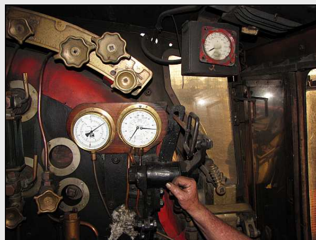
P10 – We aren't going anywhere for a bit. The short goods train has a vacuum leak and we can't get the brakes off. Attie is holding the brake lever in the run position and the ejector can't keep up. (Left half of the RHS duplex gauge.)
