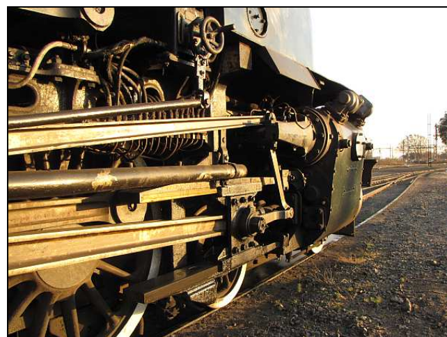
P08 – Close up of a lubricator's quarter, in this case, the right motion of the front engine unit. Although the rods got a bit rusty in storage, the oil leaks and slow siphonage from the pipes kept the working surfaces nicely oiled.
