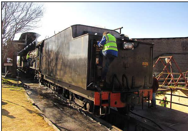
P43 – With the GMAM safely stowed away and simmering with at least few spoons of water above the crown sheet, Jeandre and Johann got busy cleaning and oiling the 12AR respectively. I caught Alan Lawton descending from placing the tender filler hose to top the tender's water level up – as this engine would be standing for another hour yet.
