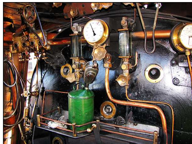
P46 – In the cab, the 12AR's pressure was a bit low after fire cleaning. The lubricator is done and it is busy warming up before the sight glasses are blown down. The left-over steam oil was being decanted back into the green can.
