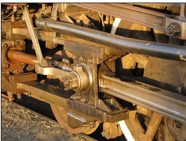
P09 – Detail of the GMAM's crosshead and slippers. The 'extra' pipe just above the cross head is a part of the 'H' shaped pipe network provided to bring in auxiliary water from dual pipe couplings fitted to the buffers at either end.
