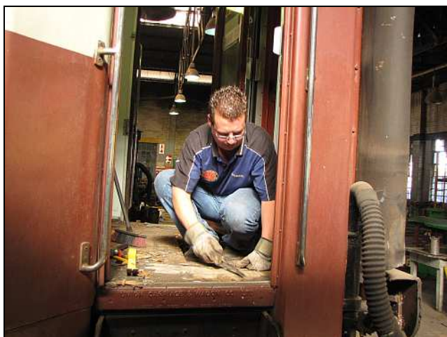
F01 – Simon Bennett is busy working at chipping away the aged vinyl sheets. SAR steel coaches do not have rubber seals on their doors, relying on the protruding lipped frames to channel the rain water at the sides, and the walkway lip as a dam. This area is quite prone to water damage.
