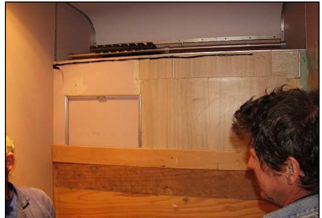
S20 – The fit-board is in place. See the colour schemes? Grey laminate = Original. Institutional green = Dave Rogers Tour 2007. Pink = Setimela. To eliminate the circus-train colour combos we currently have, the coach will be painted in neutral colours based on browns and beiges, with each Gold Class compartment done in a different tone.
