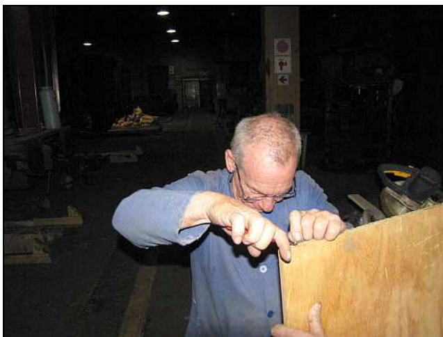
S17 – Tsk! Tsk! Using flush-cut electronic side-cutters, Gordon pulls out nails that were driven into the ENDS of that plywood sheet. It must be good stuff, as there was no evidence of splitting at the nails as you would expect.
