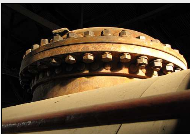
P17 – The dome gave us much trouble when the 12AR was recommissioned three years ago. This time it didn't have to be disturbed so we are confident of no leaks here. (Leaked like a sieve on 9 Feb, but one round on the nuts fixed it!)
