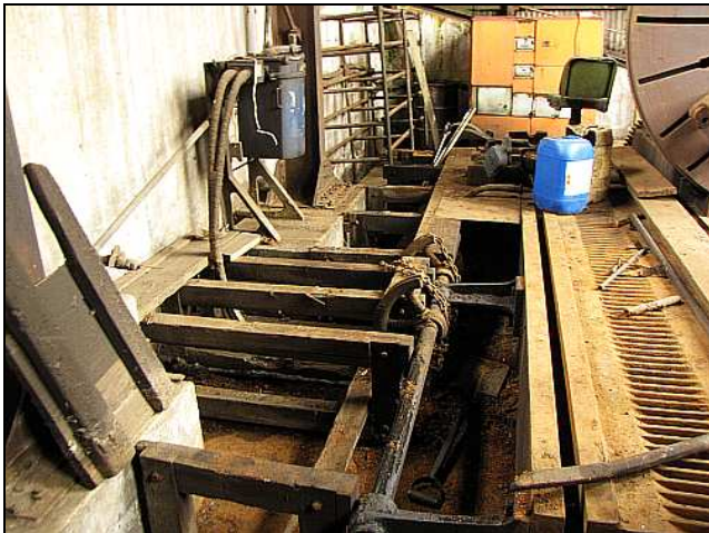
W07 – The old floor boards were lifted and decades of debris and lost tools removed. (The spade is not OEM!) The very slow moving quadrants drive lengths of chains, draped around drive ratchet clutches, which in turn slowly extend the cutting tools across the wheel profiles.
