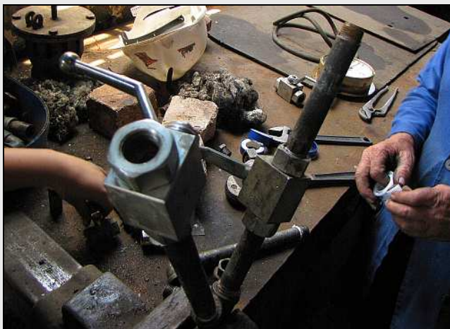
P01 – A view of the two new high-pressure ball valves mounted onto the test injection line. The old valves were cheaper plug-type valves and they were leaking under test pressures and causing false boiler-leak readings. These valves need to hold a seal of at least 1640kPa for 3 hours.
