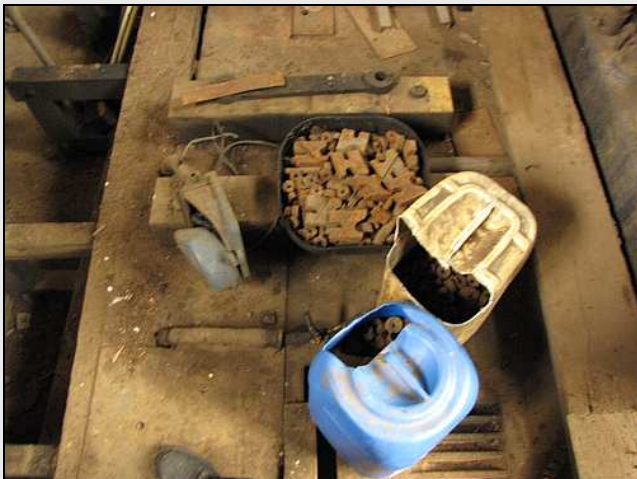
W15 – Three containers of cutting tools and accessories were recovered from under the floor boards and around the base of the machinery. Over how many decades have they been dropped through gaps and replacements have just lazily withdrawn from 'never-ending' stocks?
