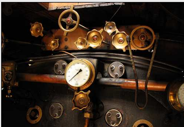
P05 – The serviced gauge in position. It has been recalibrated and certified. However, it won't receive the 'red line' blow-off mark until the boiler is steam tested and the lifting pressures of the two safety valves are set.
