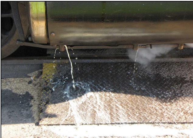
S13 – Safety hazard in the making. The residual steam oil is still running through the cylinders and is going to make that cross ramp very slippery. The steam oil actually forms a soapy emulsion in the cylinders, hence the milky colour.
