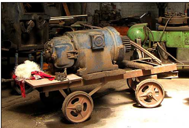
W17 – This is the wheel lathe's drive motor at the start of the project. It has recently been sent to a motor specialist for inspection and overhaul. It is likely to need new slip-ring gear and bearings, but the windings should be OK. We were lent a hydraulic palette loader for the loading job as we can't get the forklift out through the main doors.
