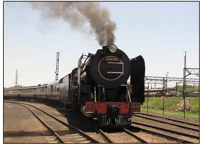
S08 – Coming to a halt at the end of the move, 15F 3046's 'scratch' fireman has just finished 'feedin' de gol'fish'. That is: a light sprinkle to keep the fire alive but not to raise steam, as 'Janine' was already thinking about blowing off.
