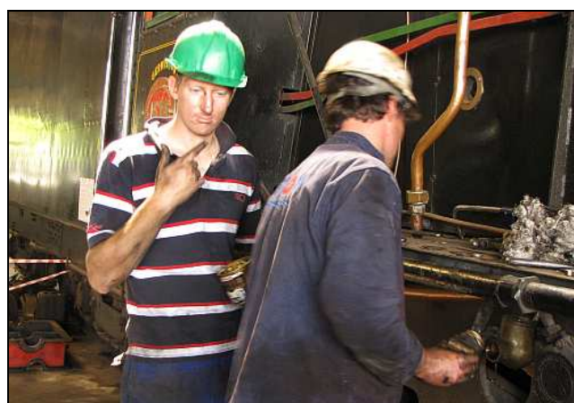
P18 – Copper Slip! Yummie! George tries it out as the slightly saner Dawie re-assembles and seals the RHS blow-down outlets. It may as well have been done even they couldn't pressurize the boiler that day.
