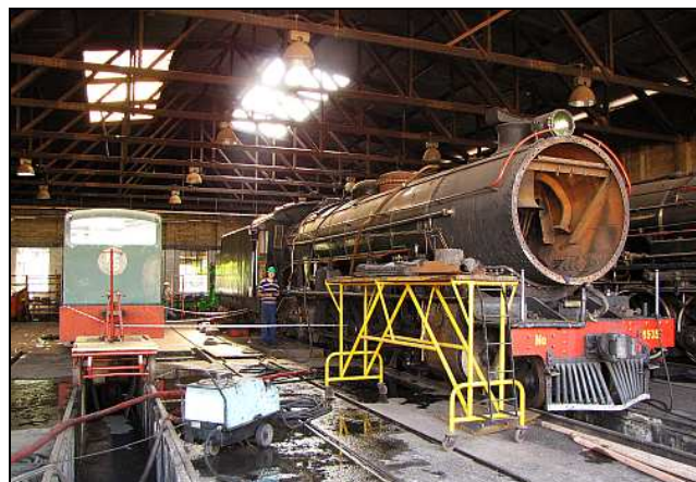
P06 – George tops up the boiler (via a hydrant) using a top washout plug hole. The blue WAP pressure cleaner in the foreground was to be used to pressurize the pre-filled boiler – but some spectacularly bad wiring shot that idea down.
