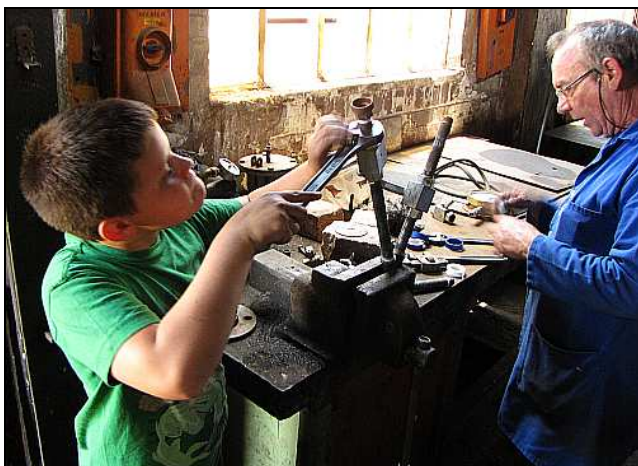
P03 – Gabriel Blore puts on his concentratin' face as he matches up the 'shifting spanner' to the pipe fitting. This would be the drain outlet. He had just been taught which way to use an adjustable spanner (Moving jaw leading into the rotation) and is happily applying his new knowledge.
