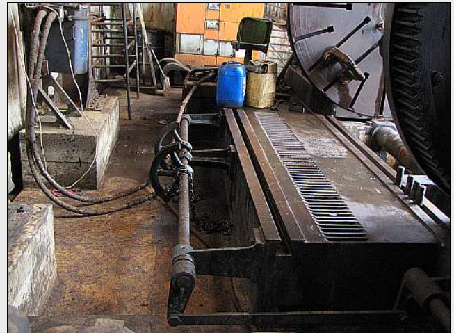
W08 – The same area a week later. The wood and floor boards have been removed. The cranks and linkages for the tool feed quadrants are now exposed. No flooring does expose the mechanical parts, but reduces the fire risk, improves drainage and reduces the risk of losing tools.
