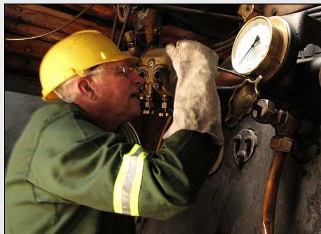
P04 – Club Secretary Stewart Currie has recently retired and will be putting some locomotive time in. Here he is just tightening the small bore steam pipe after snugging down the gauge's base ring. He wasn't sure of the gauge shut-off cock's location and would soon be doing some pipe tracing.
