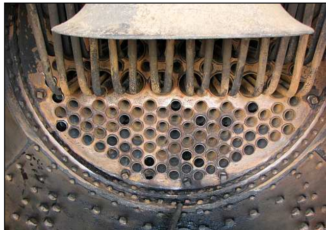
P14 – With the sealed boiler filled up to water mains pressure, there is no sign of a water leak at the recently completed front tube plate. This was between 700-800kPa. The tube plate had been labourously cleaned with a pneumatic wire brush the previous week by Jeremy Wood.
