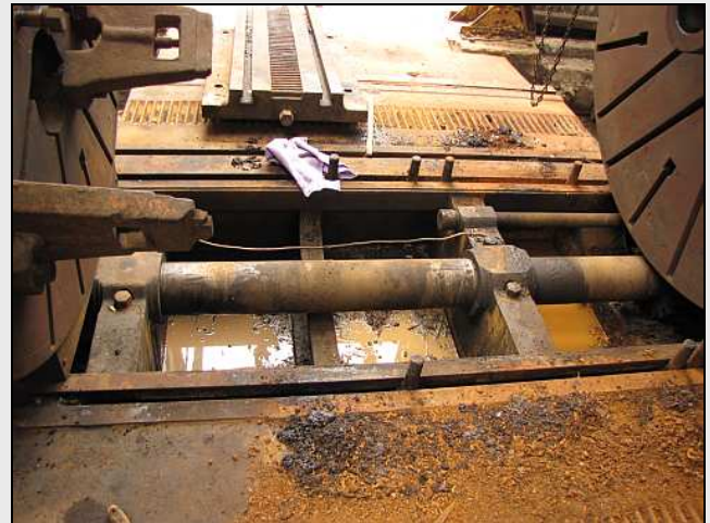
W14 – This was the state of the transfer shaft pit with the project just started. Although the lathe itself was covered in a tarp, water still got into the building through the decayed roof. Note the oil line running to the center bearing.
