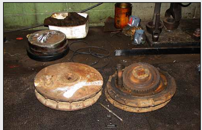
W12 – The missing tool-feed ratchet clutch (LHS) was later found amongst the junk. You can clearly see the indents where the chain links run. The chains are looped around the ratchets and are pulled at a slow rate by the quadrants. (W09) If the chains are lifted from the rims, the outer casing can be manually wound back to release the cutting tool.
