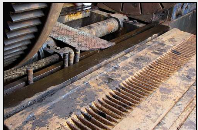
W18 – The sliding tool-stand bolts were found to be stuck. Someone had put a thick layer of bitumen into the traverse groove, probably in hope of stopping the square-shaped heads from rusting up under the old decayed roof. Coenie was tasked with cleaning up the slots – with a fun mixture of solvents, old chisels and scrapers.
