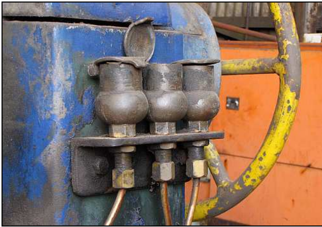
W13 – It is a minor miracle that these three oil cellars had survived intact without disappearing. Two of them even still have their wicks. These oil cellars lubricate the pedestal bearings for the drive shafts for the two chucks. The copper oil lines have since been removed for cleaning.
