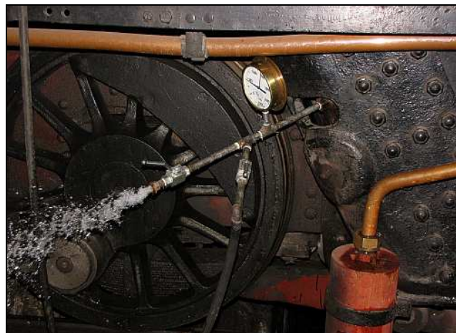
P02 – Here is the finished contraption in use a few hours later while draining the boiler. Note the boiler pressure. The lower valve is the filler line. I was sent out to purchase a tee-piece for that gauge and in classic fashion, the depot chumps had found a spare one by the time I got back. Grrr!
