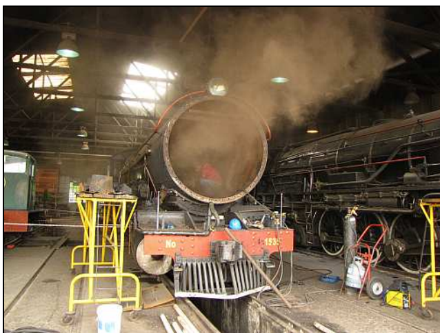
P15 – Here's what Susie's front tubeplate scrub-a-thon looked like a few weeks back with Jeremy Wood really raising the rust after the boiler boys had gotten clear. As per workshop rules, Jeremy had goggles and a facial mask on. The boiler is hydraulically tested with expanded tube ends only (rear end with copper ferrules), the rear end beading and bead-welding done afterwards.
