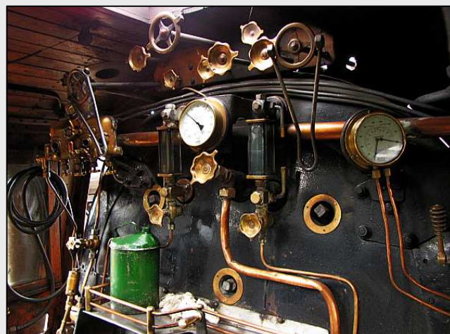
P50 – Dawie gave me the 12AR loco at just under 800 and I had given her a drink after asserting that she would not be moved. She dropped to just above 600 which is too low for safe operation of the brake ejector. I prefer to keep locos between 800-900 for the night to strike a balance between wasting steam and heat with a hot high pressure boiler, and having to thrash the boiler in the morning to get steam up.
