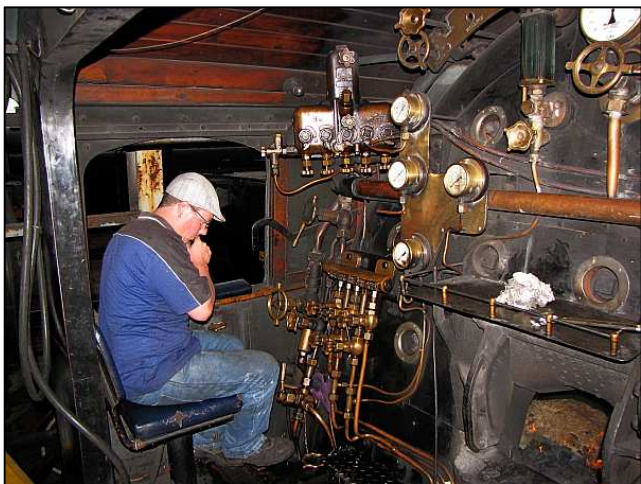
P55 – Warm and dry in the 15F cab, with a confident full-width bank of coal, Simon is kicking the injector cock back to mid-position to close it. You have to find the sweet spot slightly off-center to fully close the loose-linked valve.
