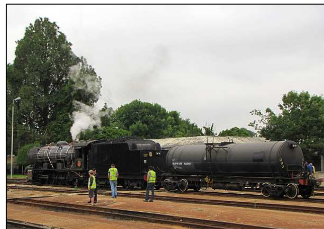
P16 – The 12AR and assorted crew members just got to hang around and watch the shunting. They weren't sure if Susie needed to be moved later, and she had raw coal on the grates anyway (From the turning operation) – which could jam the grates if it was shaken up. So the fire needed to burn down a bit.
