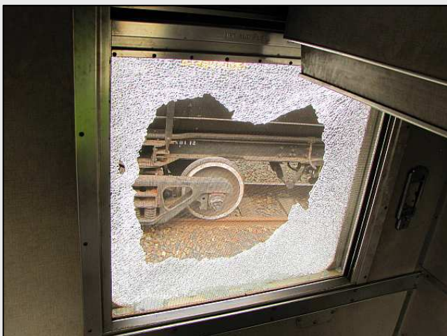
P23 – Although the caboose has seen some vandalism and is starting to lose its fittings, it is still quite restorable. But we haven't made an offer of repatriation as we don't really have a use for it. The moiré pattern effect in the photo is the still-intact insect screen over the smashed glass.
