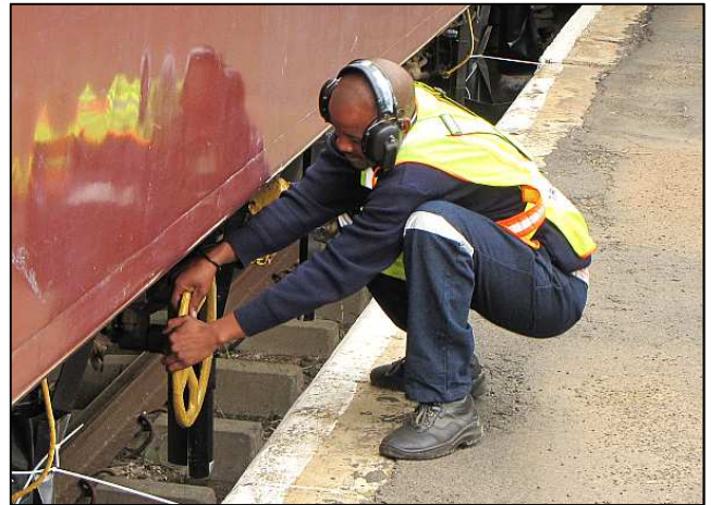
P08 – As an added touch of luxury, the TFR diesel crew even pinned the sleeper train down for us – showing their fitness and flexibility by doing it from the platform side. However, we later checked the ‘pinning’ ourselves and applied scotches. Note the neat headphone/ear muff type crew radio this young man is wearing.
