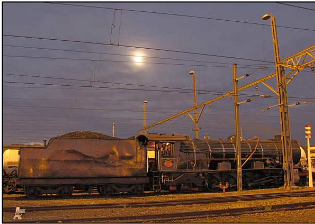
P05 – Luna the Silvery joined me and kept me silent company in the morning. ‘Susie’ the 12AR started picking up steam at about 5pm after I pushed the fire halfway forward and put a little bank at the back. We could have a good clean out at the Bethlehem MPD in just an hour or so.
