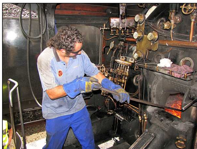
P28 – Andreas 'Bobtail' Matthee is at the hot end of this team, busy pulling the burnt-out fire back towards the open grate. He had also just joined us the day previously, along with Dawie and Johann.
