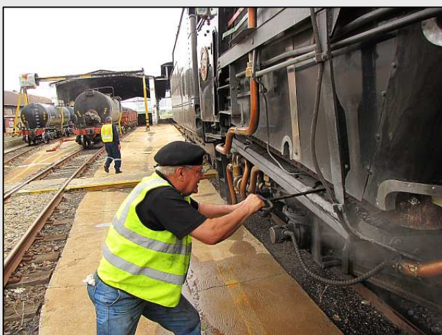
P27 – Ou Bullie-burgers is raking out the ash pan after the locomotive's second quick bunt-back to clear the ash chute from the shallow space above the sleepers. You can see three tankers ready for filling in the background.
