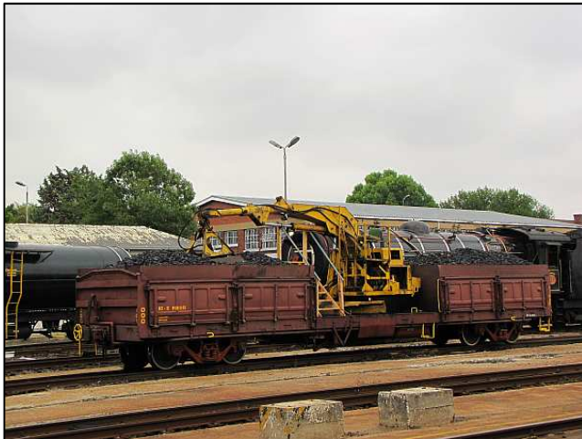
P17 – The coal handling wagon is spotted on its own for easy access, while in the background, the trio of water tankers can be seen being pushed back towards the workshop's two approach tracks.
