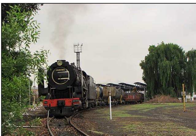
P13 – Meanwhile, both anvils had been switched pointy-ends Southwards and had been run back from the turning triangle. 15F No.3046 had been run around to the rear of the service train (cf P04), and is pulling the wagons out for shunting, leaving the day-sitter coach and caboose behind.
