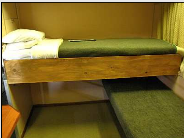
P11 – The offset bunks of a silver class compartment – as installed by a failed tourism company. Although the bed rails are too deep and the finish is amateurish, the design permits headroom and easier climbing into the upper bunk.
