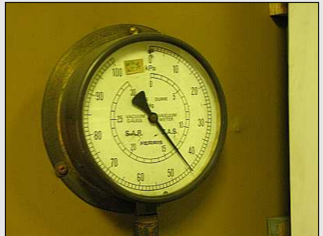
P38 – Transnet Traction frequently has trouble with vacuum exhausters as they are being used less and less. We aren’t doing too bad here, although they tended to start the train moving with the rearmost brakes still applied. Lotsa squeal!
