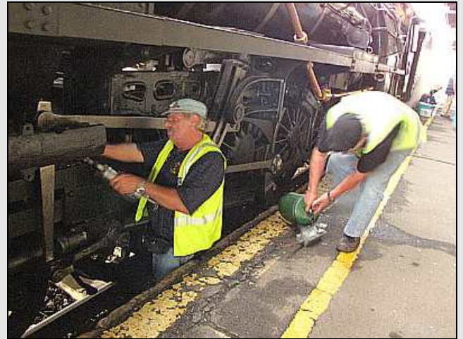
P54 – Not the safest of jobs at jobsite, but it has to be done. ‘Cupcake’ Le Roux does the greasing. Note that fireman Johann is using a home-made rectangular-bodied oil feeder for the slippery stuff.
