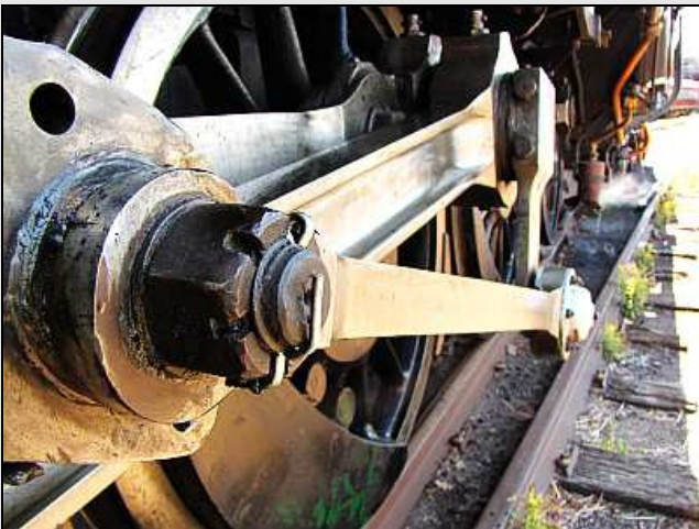
P07 – The rods had been cleaned during a busy short week. In the foreground is the stained and SAR fitter-battered ear of the expansion link and we are looking along the gleaming angled length of the eccentric rod.
