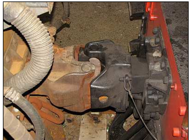
P52 – Even the Reefsteamers Janney couplers look well-kept. What I found interesting here was that the steam locomotive, with a longer rigid wheel base, has a shorter coupler shank than the pivot-bogied Class 6E1.
