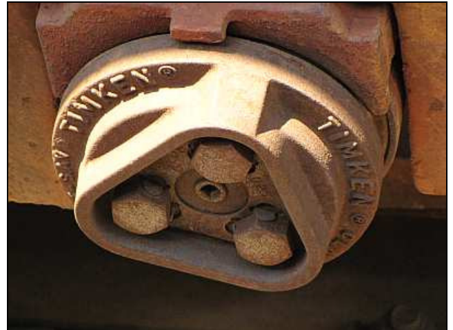
P24 – Close up of a Timken bearing set in the wagon repairs line. Note how the three hex nuts for the cover are safety-tabbed into place.
