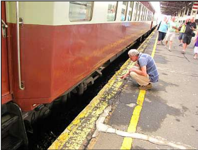
P59 – Back to sniffing bogies and playing patty-cake with the axle bearing caps. Apart from the slightly tardy brakes, no mechanical problems were found. Checking the other side is more fun in close proximity to the toilet scat pipes.
