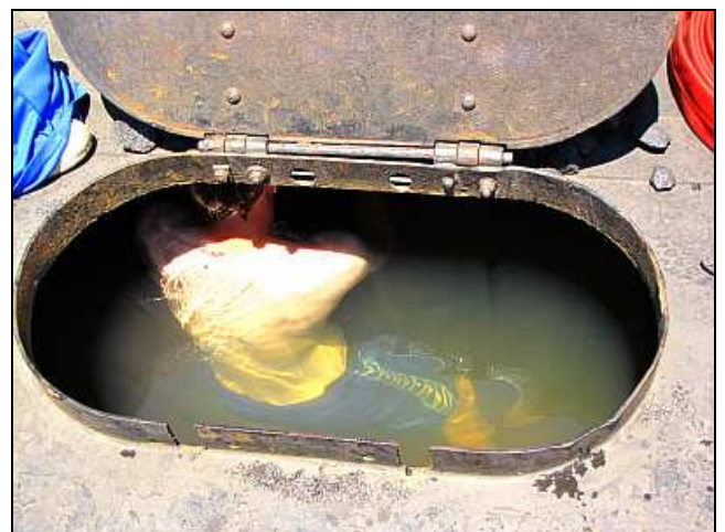
P04 - Wett-Nutts takes another dive. We had to get that plastic bag out of there otherwise it would get sucked into the injector's water inlet and block the works. They never did find that bag and shut the tender's baffle gates instead.
