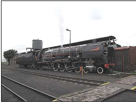
TU10 – The steam locomotive equivalent of ‘one for the road.’ Elize gets a tender top-up from the parachute tank and this will be the last drink until arrival and shunting at Boksburg East that evening. The first of the four safeties have lifted again – this one is the one of the two Ross-pop type valves.
