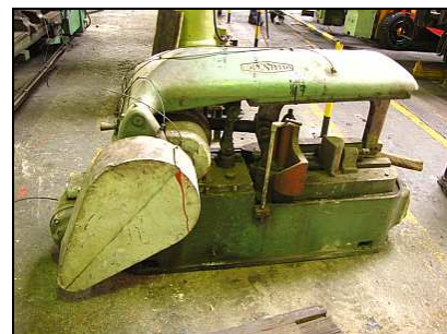
The Wicksteed saw in a safe temporary location. The object protruding from the right is a block of wood inserted to protect the saw blade.
