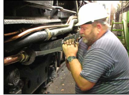
In one of his first tasks around the Depot, Robbie comes to grips with the ash pan cooler supply unions on the Class 25NC No.3472 'Elize.'
