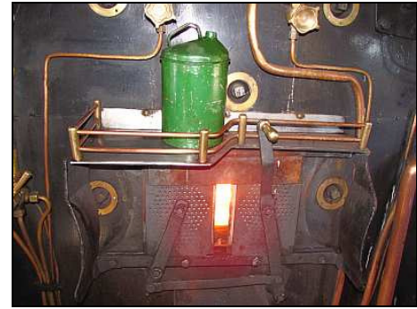
A winter-night-cold can of Compounded Steam Oil ('Valve Oil') being heated on the Class 12AR's flame plate to render it fluid enough for easy pouring.
