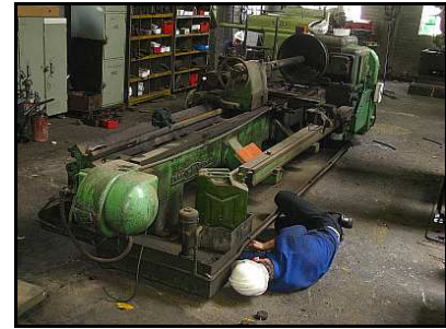
Patrick Ackerman adjusts the feet of the lathe to get it to stand stable and level.
